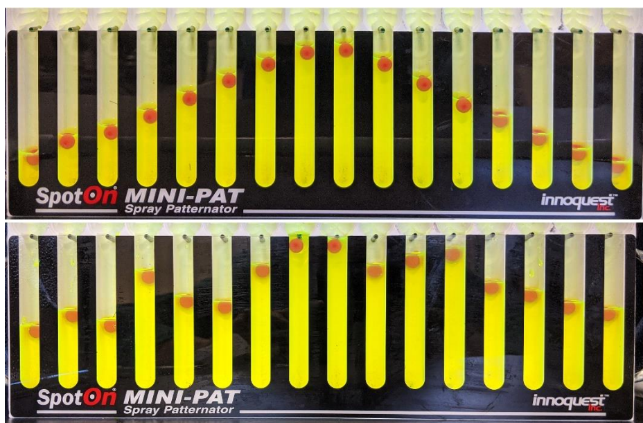
Figure 3. When testing the new versus worn nozzle, the pattern may show irregular output patterning. The new nozzle (top) compared to a similar nozzle used after one season of heavy sulfur applications (bottom) shows very different output pattern. Photos by Margaret McCoy, Washington State University.
